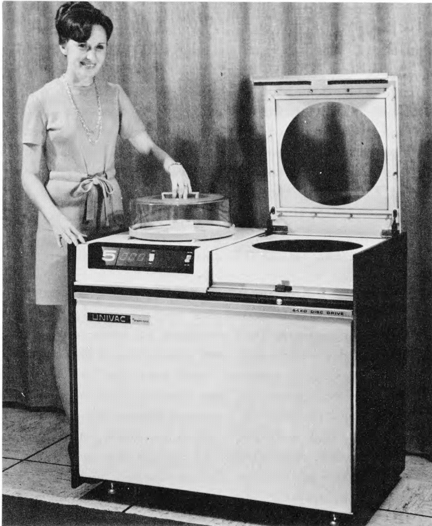
Figure 1.6 Univac 8440 Disc Drive (Courtesy of Sperry Univac, A Division of Sperry Rand Corporation)
